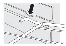
To refit the shelf, line up the shelf with a groove in the oven side and push the shelf back until the ends hit the shelf stop. Lift up the front so the shelf ends clear the shelf stops, and then lower the front so that the shelf is level and push it fully back.
